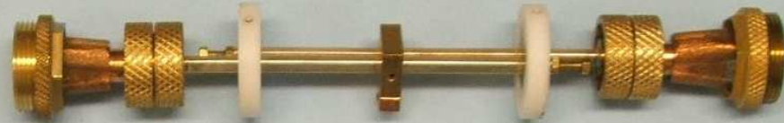
Band-pass filter (WR-05) for removing thermal radiation complete with coupling horns to overmoded waveguide (WR-28)
