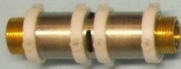
Thermal break in fundamental mode waveguide - two back-to-back waveguide tapers (WR-05 to WR-28) with needle point mountings
