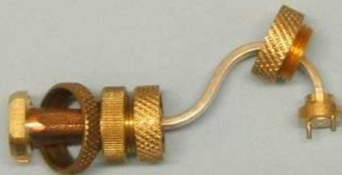
Fundamental mode 'Swan-Neck' coupling piece for microwave cell
